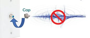
Use terminating caps provided by FOCUS Broadband on any open coaxial wires to block noise from entering the circuit that has the internet signal. Attach the caps to all unused outlets.
