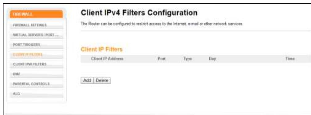
Figure 49: Set up client IP filters screen
