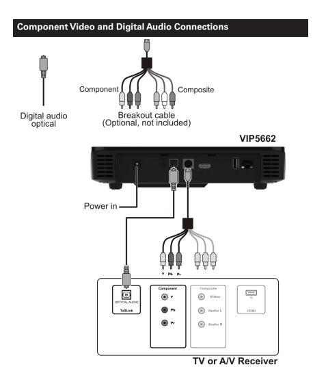
If you use a DVI video input to connect to your TV, you will need to provide a separate connection for the audio. Use the OPTICAL S/PDIF output, which offers digital audio quality, including support for Dolby Digital 5.1 Surround Sound.
