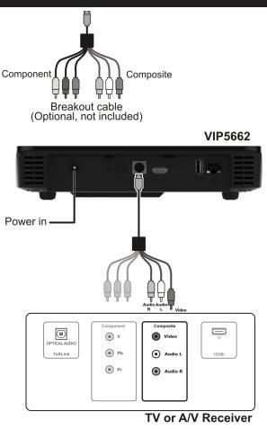
If your HDTV has composite video and analog stereo inputs, connect the composite outputs using a Breakout cable to the correct inputs on your HDTV (as shown).
