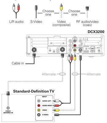
Note: S-Video and Composite video require separate audio connections. Note: Only (1) video connection and (1) audio connection is required. Note: Solid lines indicate optimum connections.
