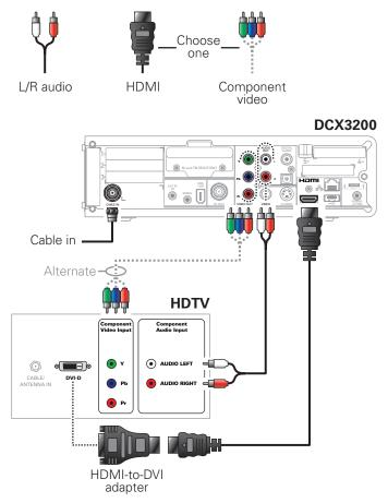
Note: Only (1) video connection and (1) audio connection needs to be made to an HDTV.
