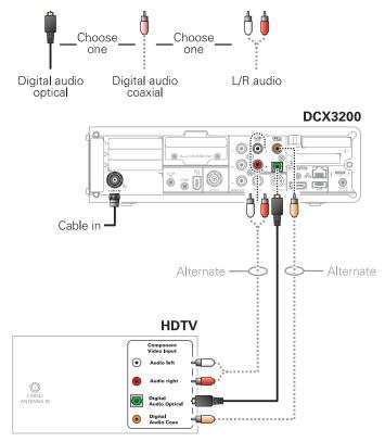
Note: Only (1) audio connection needs to be made. Note: Solid lines indicate optimum connections.
