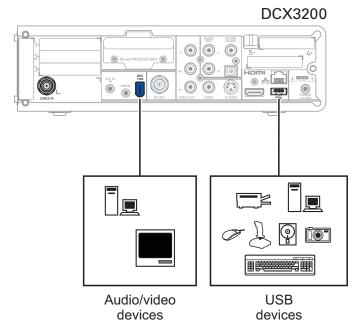
Note: Do not attempt to connect data devices without contacting your service provider. Advanced data features require the proper application and network infrastructure to operate.
