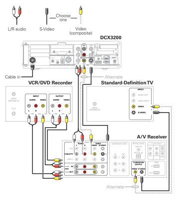
Note: Solid lines indicate optimum connections.
