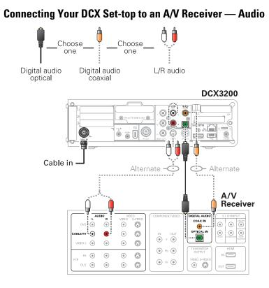
Note: Only (1) audio connection needs to be made to an A/V Receiver. Note: Solid lines indicate optimum connections.
