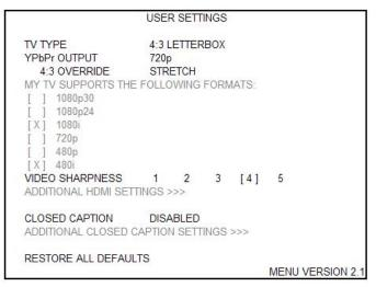
An example of the User Settings menu when the HDMI output is not connected.
